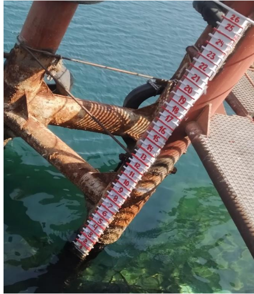
Figure 2. Tamasa is used to measure the water level at the Sea Hydrometeorological Station of the “Neft dashları” in the Caspian Sea
